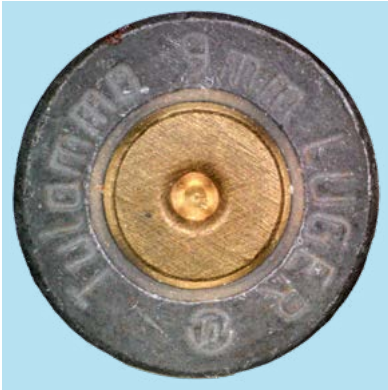
9 mm Luger cartridge case produced by Tula Cartridge Works (Russian Federation), year of production unknown
