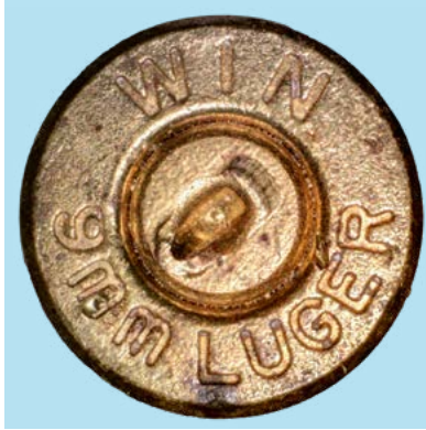
9 mm Luger cartridge case produced by Winchester (United States), year of production unknown
